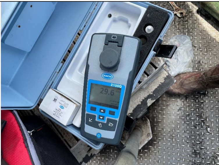
Photo 4: 1200 Turbidity Reading of 29.6 NTU.
